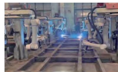
Carbon Steel Frame Welding
