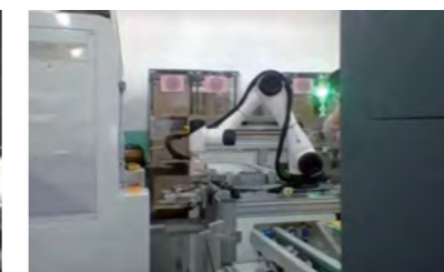
Glue Spraying Machine Loading/Unloading
