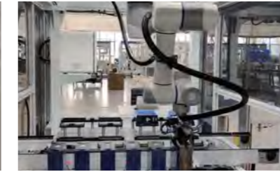
Battery Testing Loading and Unloading
