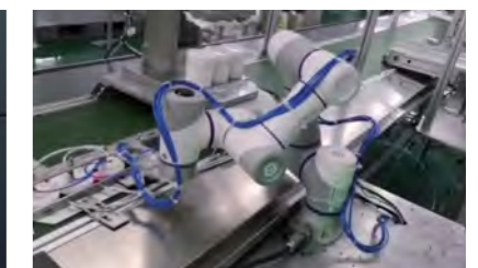
Plastic Lid Loading/Unloading
