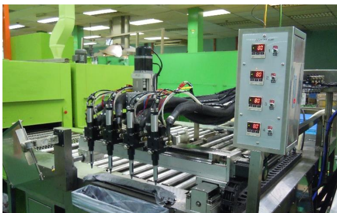
(Potting station, 4 valves)
